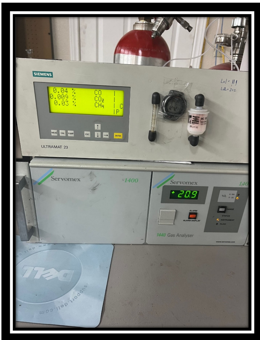
FIGURE A4 - SIEMENS ULTRAMAT METHANE, CO 2 , AND CO (TOP) AND SERVOMEX 1400 OXYGEN (BOTTOM) ANALYZERS USED IN TESTING
