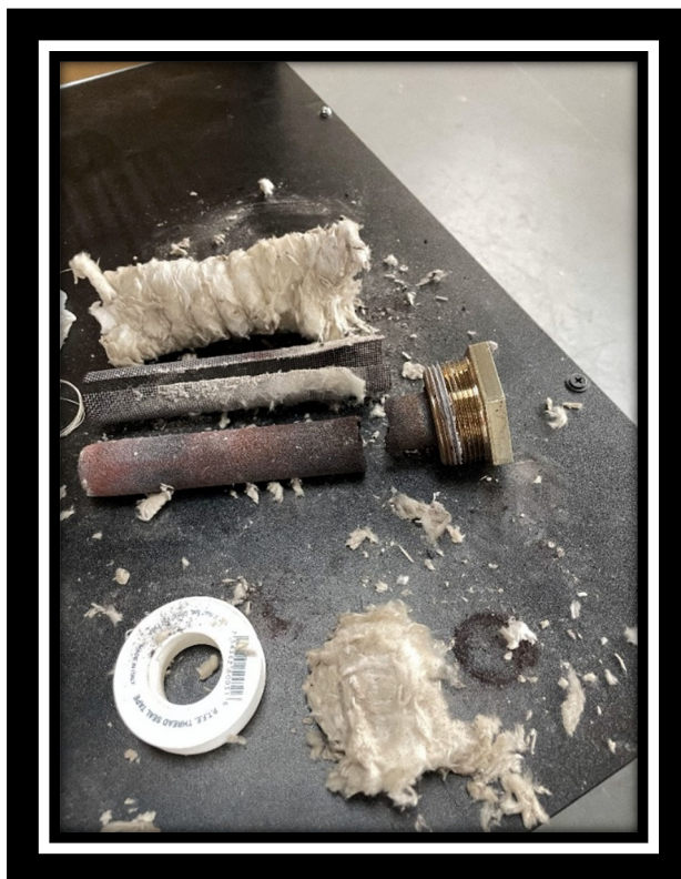
FIGURE 7.2 CATALYTIC DEVICE DAMAGED DUE TO EXCESSIVE BTU THROUGHPUT
