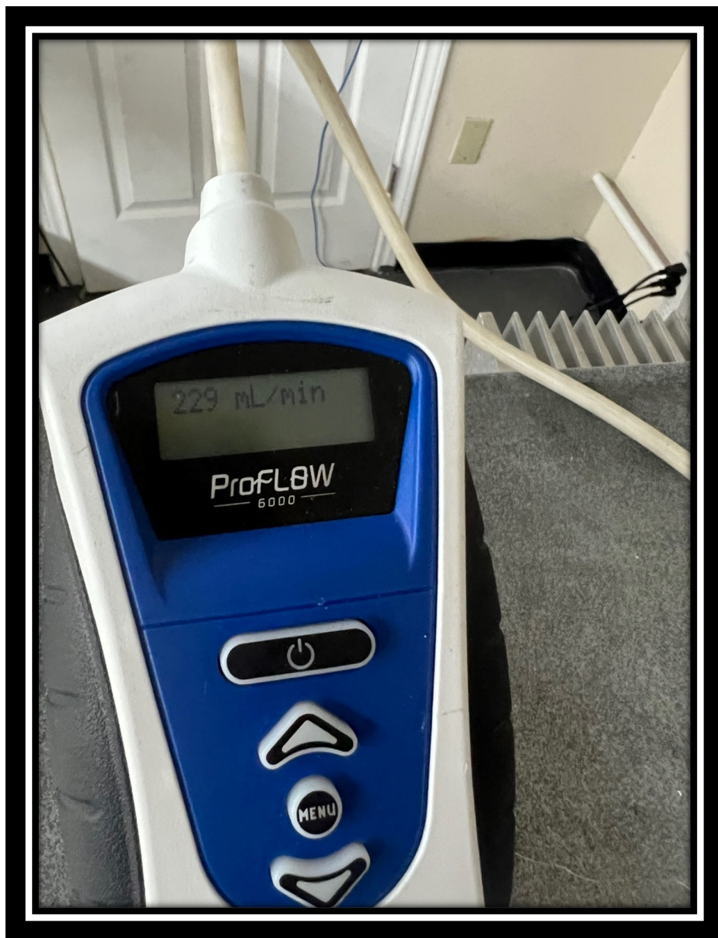
FIGURE A6 - ELECTRONIC FLOW METER USED TO MEASURE TEST GAS SENT TO TRACE TECHNOLOGIES CATALYTIC DEVICE
